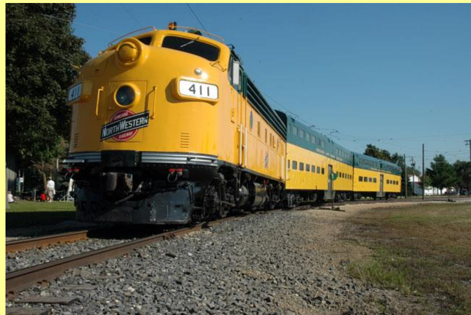
C&NW 411, an EMD F-7A, at the Illinois Railway Museum with two C&NW bi-level coaches. Picture was taken on 08/30/07 by Dave Hawley .
